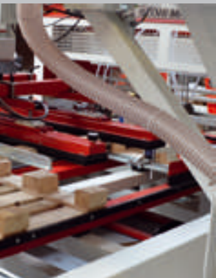
SMPT 2 - detail on a nailing machine with bottom board manipulator
