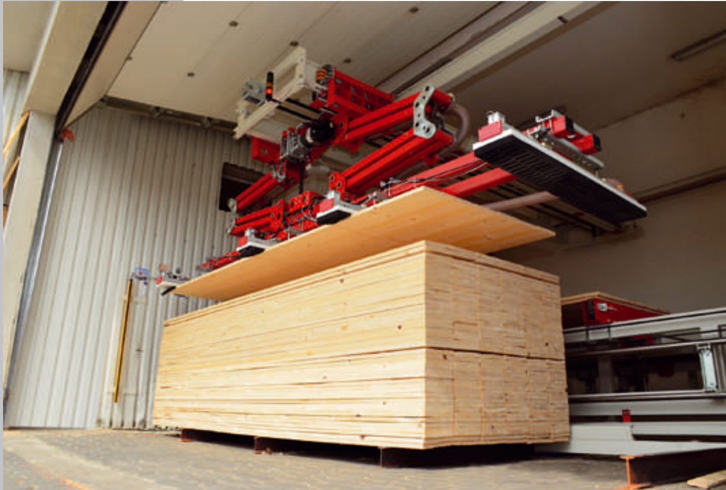
Vacuum handler with a cap scraper for the KP 900 EASY CUT OPTIM machine.
